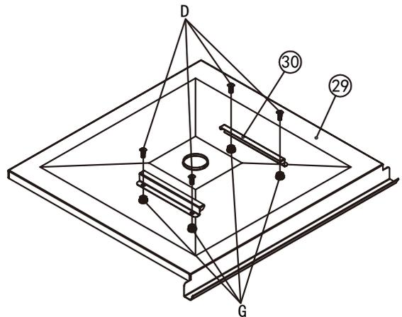
Assemble the grease cup brace (30) to the grease tray (29) with 4 bolts (D) and 4 nuts (G).
