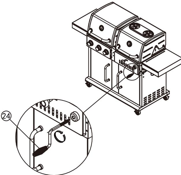
Screw the lifting handle (24) to the control panel twist clockwise.
