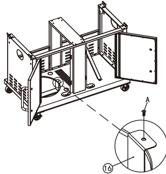
Install tank base lower (16) to the bottom shelf with 2 bolts (A).
