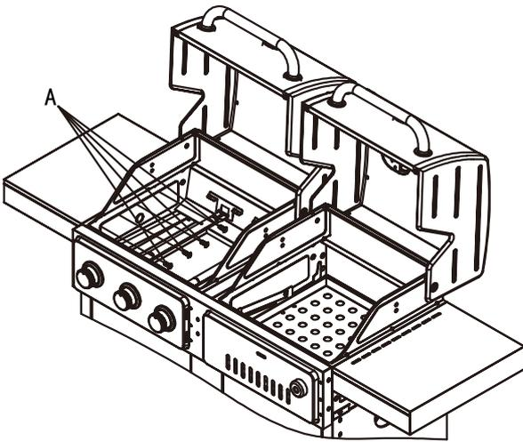
Fasten the side tables from the inside of the fireboxes with 8 bolts (A).
