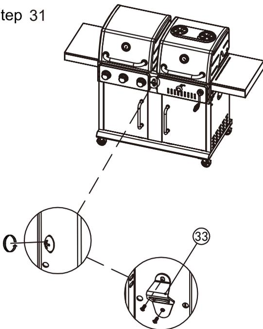
Loosen 2 bolts of the middle of control panel, fasten the bottle opener (33) to fireboxes, screw back the bolts as shown.
