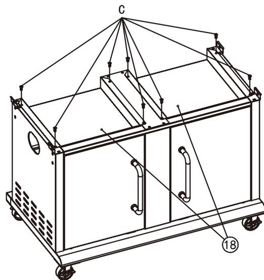
Assemble the thermal baffles (18) to the firebox brace and middle brace with 8 bolts (C) as shown.
