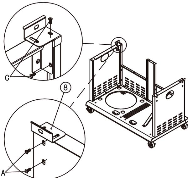
Assemble the left firebox brace (8) to the shown positions of side shelf with 2 bolts (A) and 2 bolts (C).
