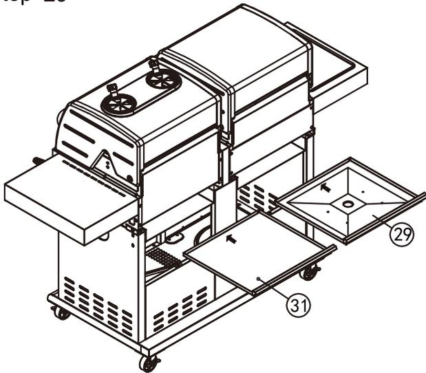
Slide the ash pan (31) and grease tray (29) underneath the fireboxes.
