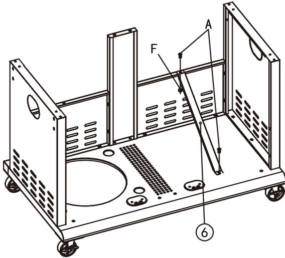
Fasten the LP barrier bar (6) to the bottom shelf with 1 bolt (A) and to the rear shelf with 1 bolt (A) and 1 nut (F).
