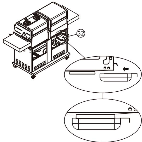
Attach the grease cup (32) underneath the grease tray.
