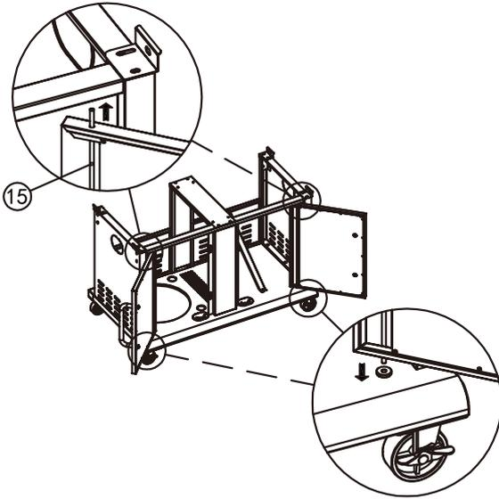
Slide the door axles (15) to doors, install them to the cart front beam and bases.
