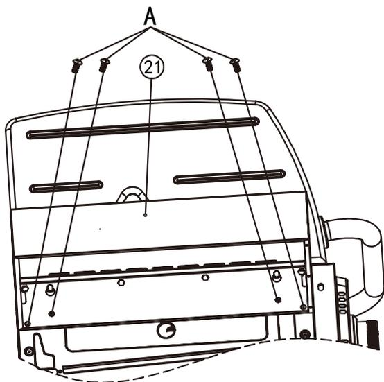
Assemble the side table (L) (21) to the firebox by hanging it to the half screwed bolts, fasten it with 4 bolts (A). Then secure the half screwed bolts.
