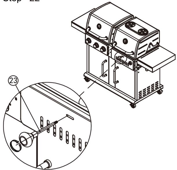
Screw the airvent handle (23) to the control panel twist clockwise.
