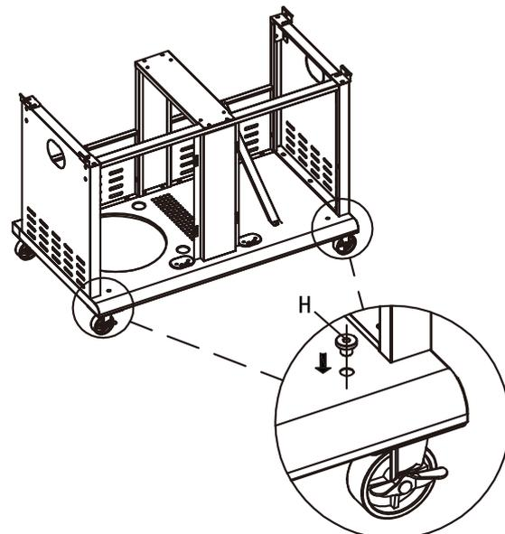
Insert the bases (H) to the bottom shelf as shown.
