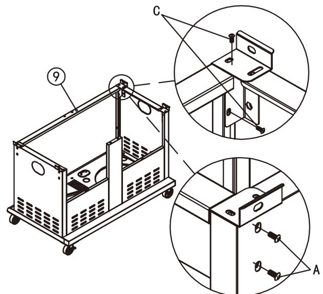
Assemble the cart front beam (9) to side shelves with 4 bolts (A) and 4 bolts (C).
