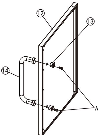
Assemble the door handles (14), handle bases (13) to the doors (12) with 4 bolts (A).
