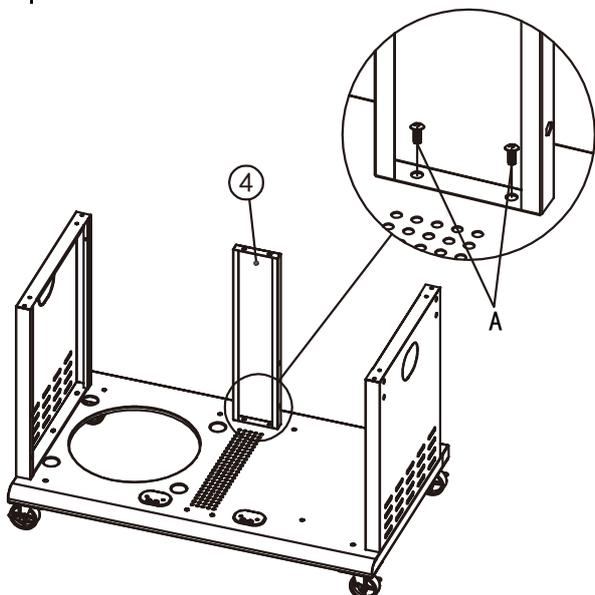
Assemble the back support (4) to bottom shelf with 2 bolts (A).
