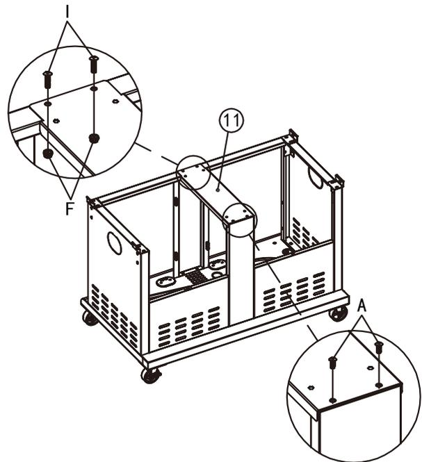
Assemble the middle brace (11) to cart front beam with 2 bolts (I) and 2 nuts (F) and to back support with 2 bolts (A).
