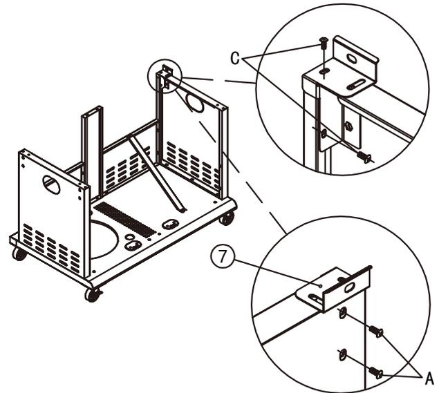
Assemble the right firebox brace (7) to the shown positions of side shelf with 2 bolts (A) and 2 bolts (C).
