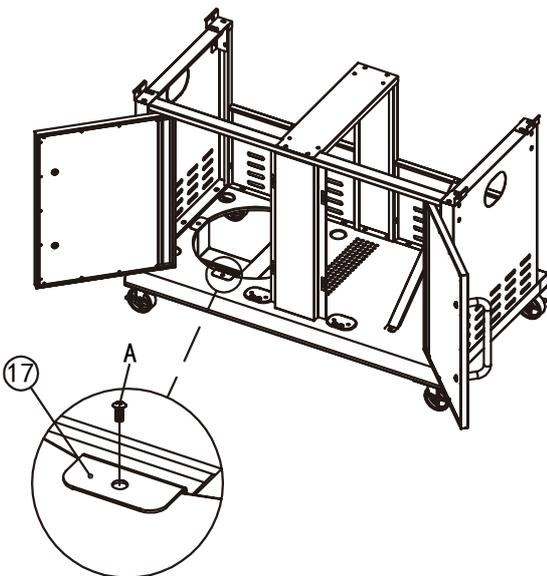
Install tank base upper (17) to the bottom shelf with 2 bolts (A).
