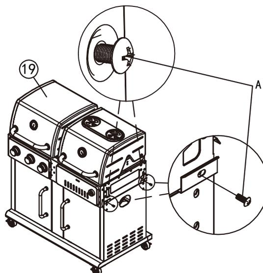
Place the firebox (19) onto cart the braces with 4 bolts (A). Half screw 4 bolts (A) to shown positions of both sides of firebox.
