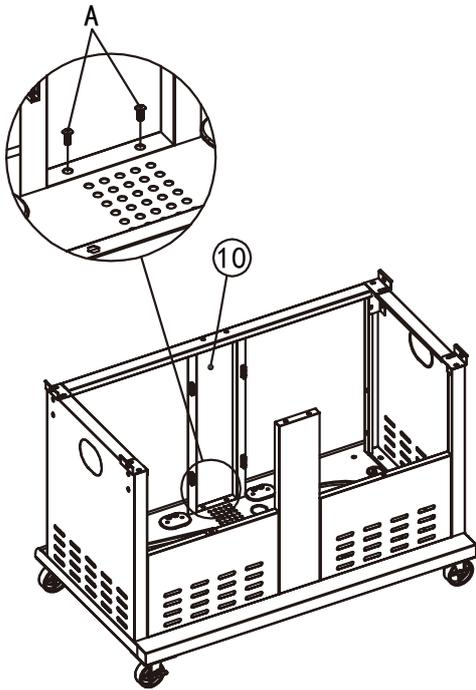
Assemble the front support (10) to bottom shelf with 2 bolts (A).
